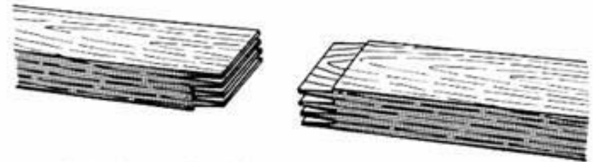
34-16. The finger joint is considered the most important industrial joint.
