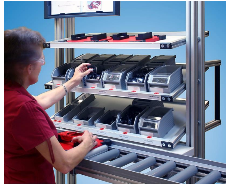
Example of manual assembly line
