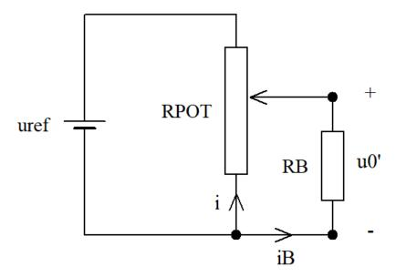
Let's denote the resistance of the entire winding of the potentiometer as  $R_{POT}$ . This resistance can range from 10  $\Omega$  up to 1 M $\Omega$ . The resistance of the winding between the ground terminal and the slider terminal is denoted as  $R_{\Theta}$ . The rotation angle of the motor  $\Theta$  j is the angle between the slider and the ground.
