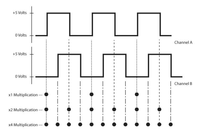
The first option is to use only one of the two channels and count pulses at the transition of the signal from 0 to 1. This yields one pulse per channel period. The second option is to use both channels and count pulses at the transition from 0 to 1. This yields two
