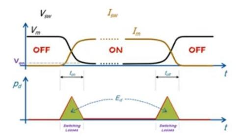
As evident from the above figure, for simplification in calculating the transition between the closed and open states of the switch, we approximate it with a linear form. Consequently, the graph for the power consumption over time exhibits two segments in a triangle and one segment with a constant value.
