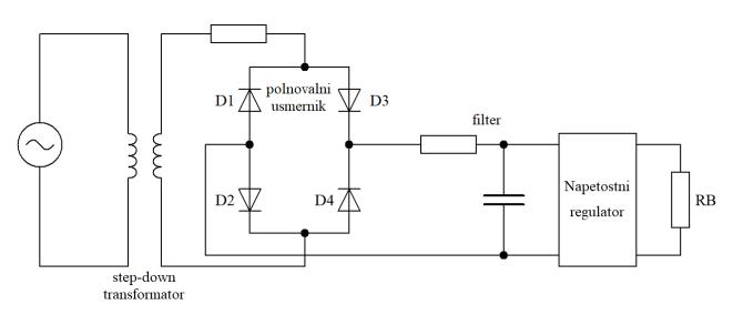
The first component is usually a step-down transformer. The grid voltage is high (approximately 330 V amplitude), so we need to adjust and reduce it by at least one
