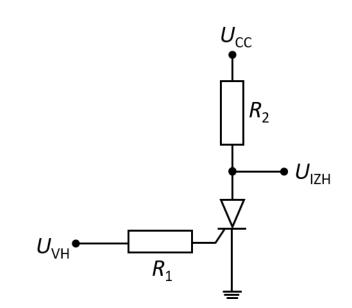
Data:  $U_{CC} = 15 V$   $R_1 = 1 k\Omega$   $R_2 = 100 \Omega$   $U_T = 0.7 V$   $I_T = 7 mA$ ,  $I_H = 6 mA$  $U_{OUT-OFF}, U_{IN-ON}, U_{CC-ON} = ?$
