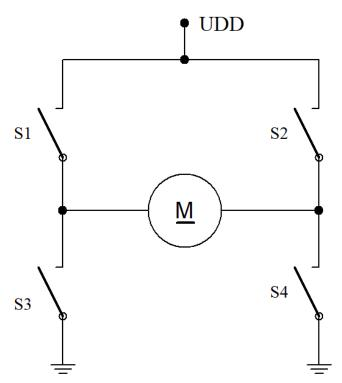
From the simplified diagram, it is evident that to achieve the desired motor rotation or specific current direction through the motor, we need to close two of the four switches
