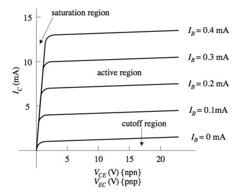
In the cut-off region, no current flows through the transistor, so it functions as an open switch. This state is achieved when the voltage between the base and emitter (V\_BE) is lower than the diode's forward voltage drop. The junction between the base and emitter acts like a diode, requiring a sufficiently high voltage to conduct current. For silicon-based transistors, this voltage is approximately 0.7 V.
