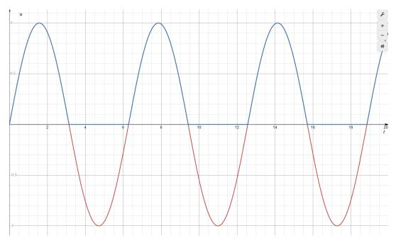
Nevertheless, let us calculate the voltage across the motor during the half-cycle of the input (grid) signal when the diode is forward-biased and conducting current. If we simplify by assuming we have a diode with ideal resistance  $R_D = 0 \Omega$ , we can determine that resistors  $R_2$  and  $R_M$  are connected in parallel. Since we are interested in the voltage across the motor, we use the voltage divider equation:
