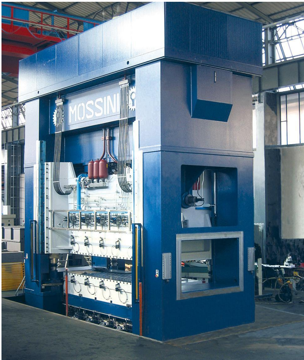
Figure 4.6 – MOSSINI 4-column hydraulic press, model PO 1500 (15 000 kN)
