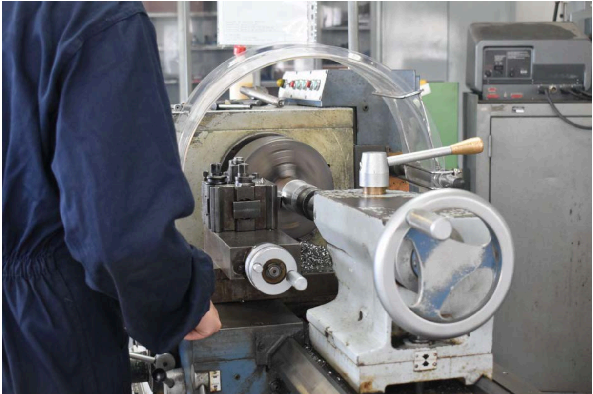
[Fig.24] Processing and monitoring phases of the mechanical piece on the parallel lathe.
