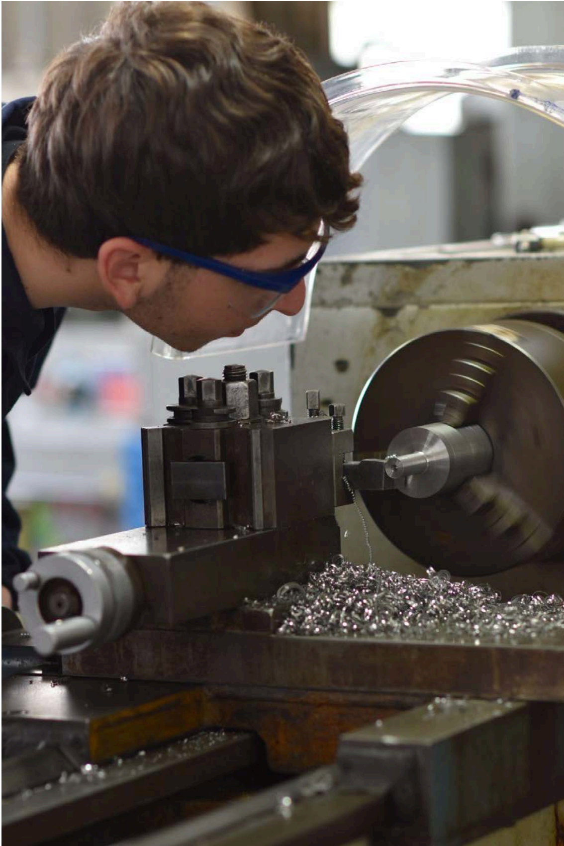
[Fig. 25] Technical Institute student during turning operations for the production of the component in the workshop.
