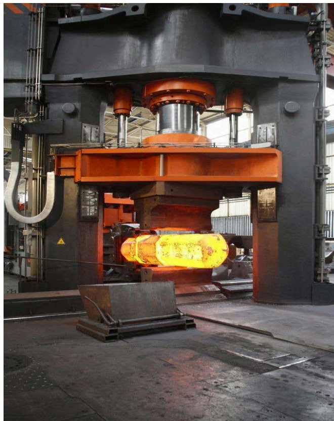
[Fig. 32] Example of a 400-ton hydraulic press for hot forging and stamping operations of steel components.
