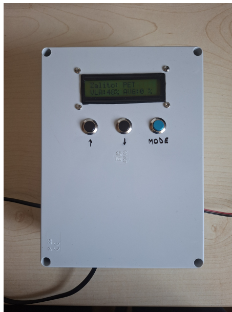
Figure 5.1: Electronic enclosure of the product
