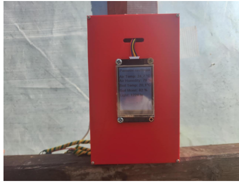
Figure 18: HMI display after installation in the greenhouse
