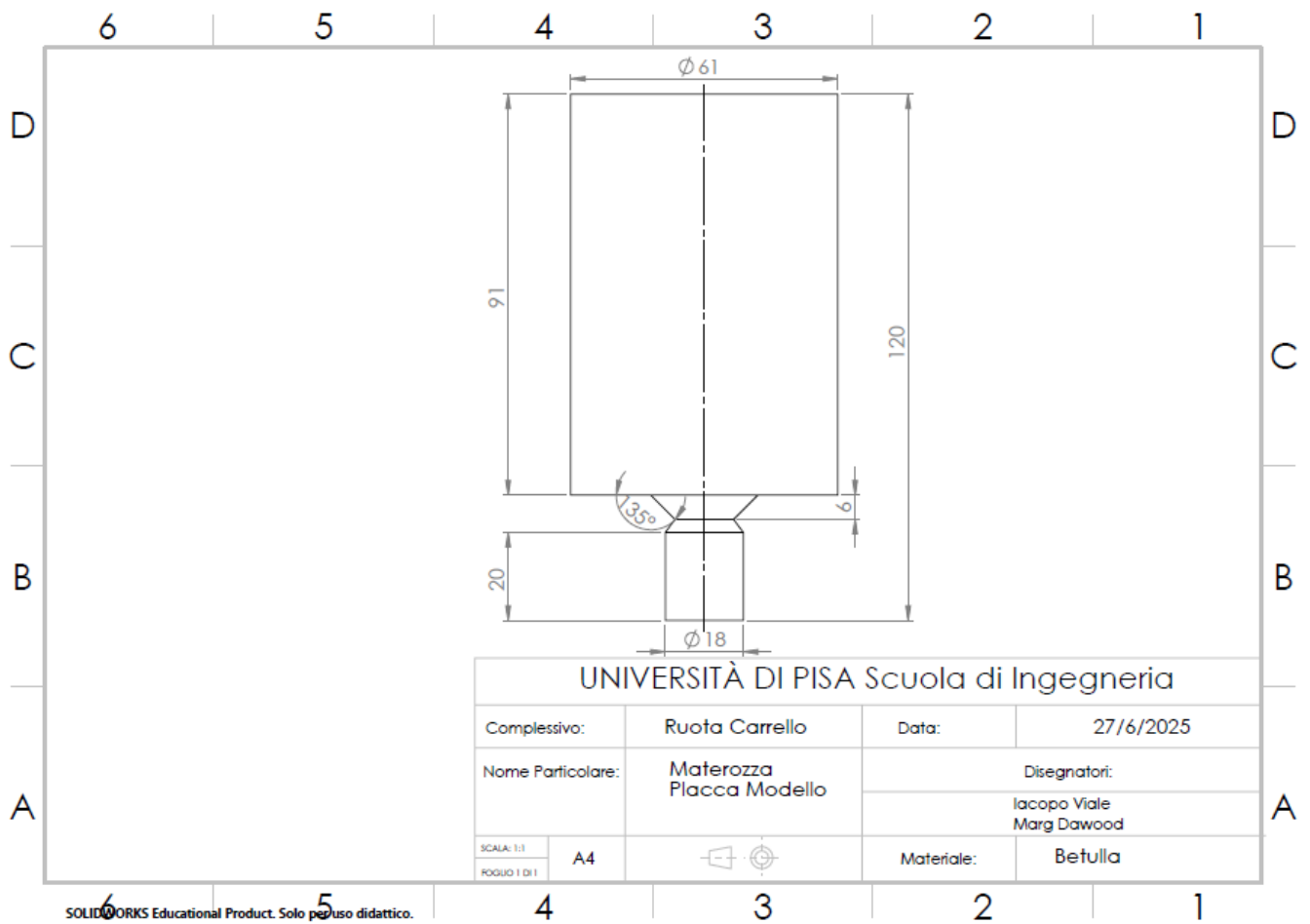
Figure 24: technical drawing "Feeder pattern plate"
