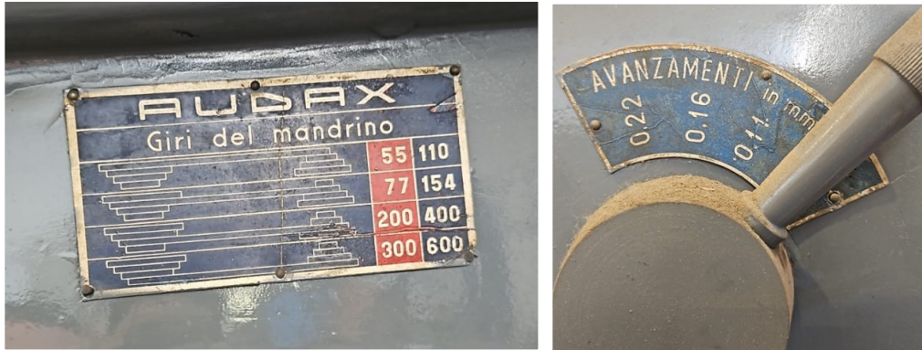
Figure 42: plates with spindle indexing and feed increments
