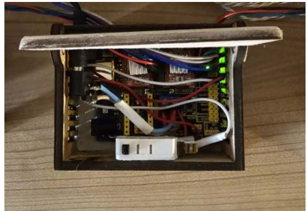
Figure 18: Finished enclosure with Arduino and G1 switch installed
