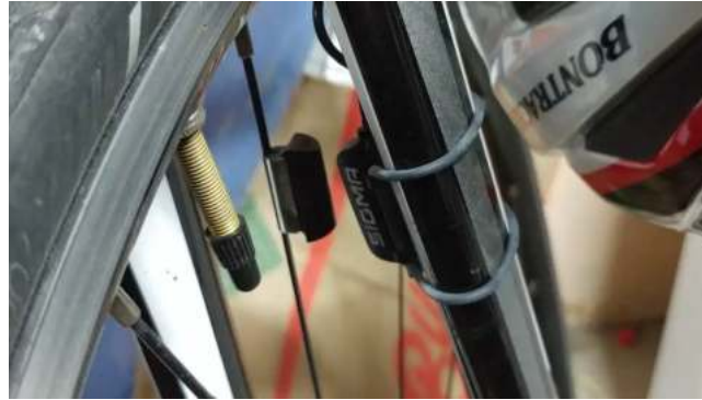
Figure 8: Reed switch used by bike computer to count revolutions of wheel [4]
