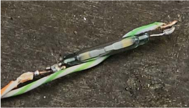
Figure 13: Reed switch before it was inserted into protective tube
