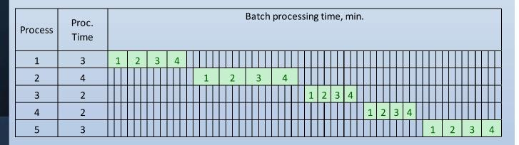
The serial production flow can be presented in the form of a Gantt chart. The times of successive processes are given. The times of all transport operations are 1 minute.
