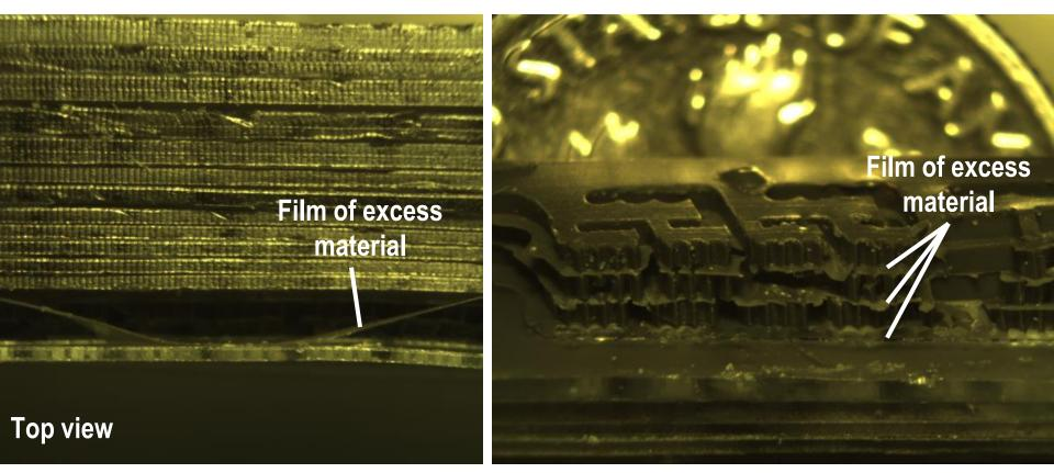
Cast material: Bi-component Platinum catalyst Silicone from Dow Corning Sylgard 170 Degassing in vacuum @ 26" Hg for 30 minutes (working time)
