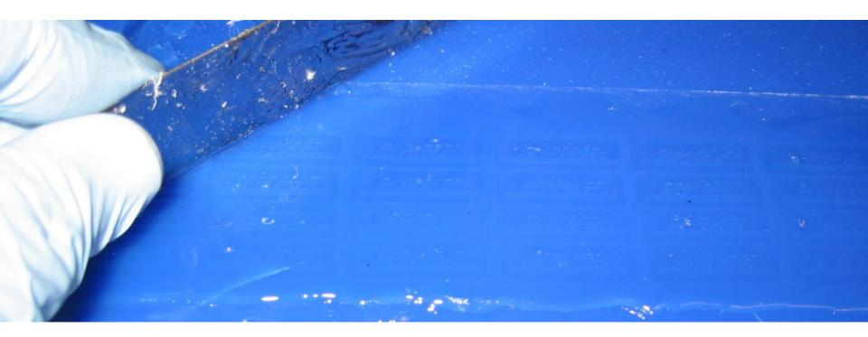
Cast material: Bi-component Urethane from SmoothOn Task 9 Degassing in vacuum @ 26" Hg for 5 minutes (working time)
