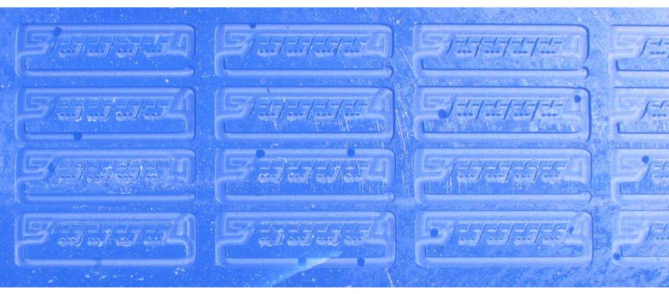
Depth of cavity: 750 µm (top two rows); 500 µm (bottom two rows)
