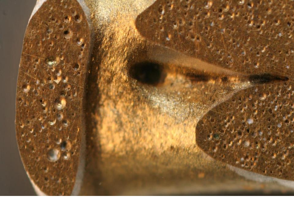
Sample Section. High porosity. Bimodal Pwd+AuSn. Inf. Temp.: 394°C
