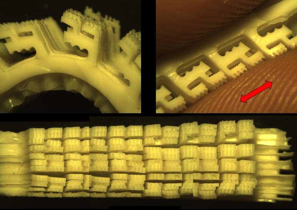
MOLD SDM Cast material Bi-component Platinum catalyst Silicone: Dragon Skin, Dow Corning Working/Cure time [min./h.]: 20/5 Shore hardness [MPa]: 10A Tensile strength [MPa]: 3.3 Elongation [%]: 1000 Degassing in vacuum @ 26" Hg
