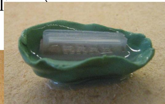
Cast material: Bi-component Platinum catalyst Silicone from Silicon Inc./Innovative Polymers P-20
