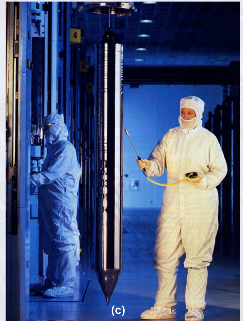
Figure 11.24 Two methods of crystal growing: (a) crystal pulling (Czochralski process) and (b) the floating-zone method. Crystal growing is important especially in the semiconductor industry. (c) A single-crystal ingot produced by the Czochralski process. Source: Courtesy of Intel Corp.
