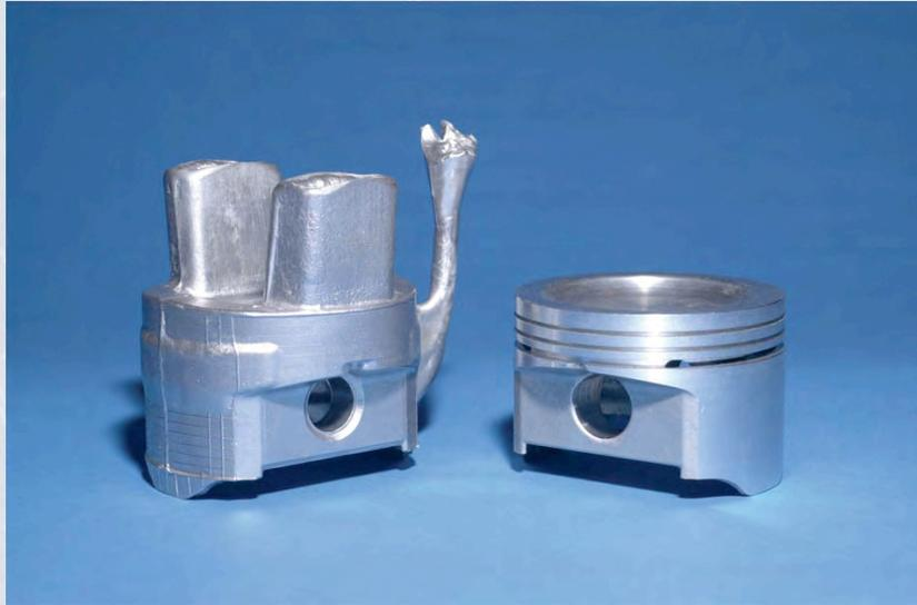
Figure 10.16 Aluminum piston for an internal combustion engine: (a) as-cast and (b) after machining.
