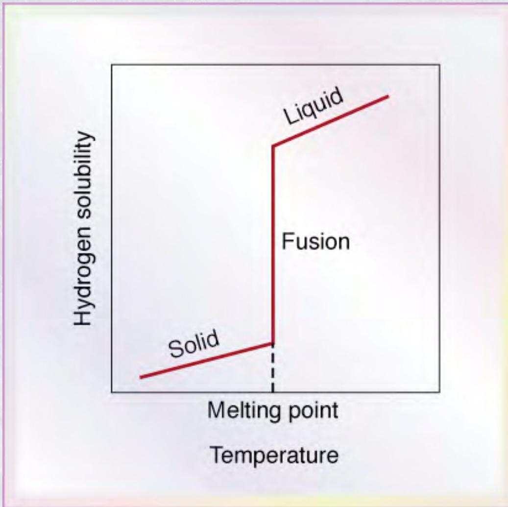
Figure 10.15 Solubility of hydrogen in aluminum. Note the sharp decrease in solubility as the molten metal begins to solidify.
