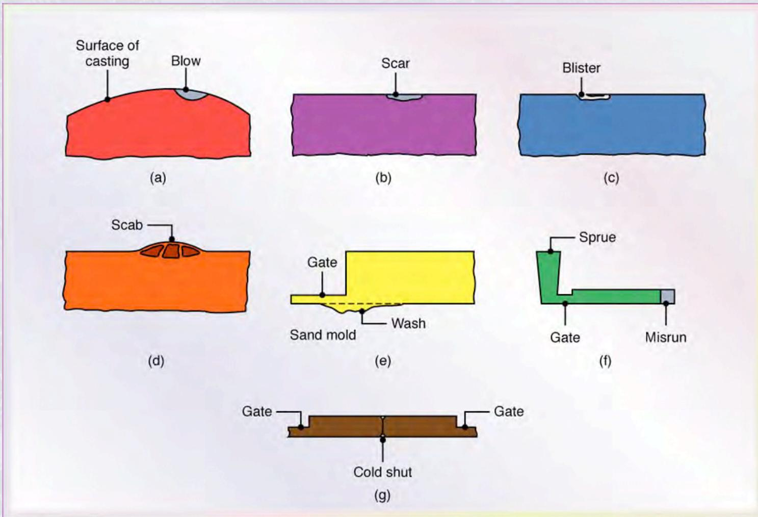
Figure 10.13 Examples of common defects in castings. These defects can be minimized or eliminated by proper design and preparation of molds and control of pouring procedures. *Source:* After J. Datsko.
