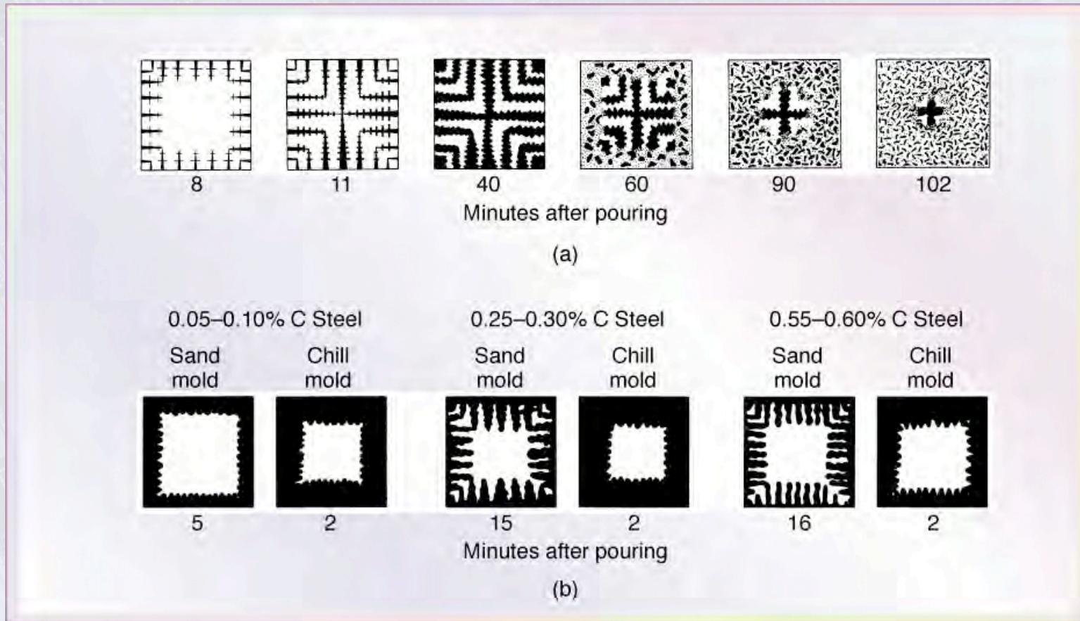
Figure 10.5 (a) Solidification patterns for gray cast iron in a 180-mm (7-in.) square casting. Note that after 11 minutes of cooling, dendrites reach each other, but the casting is still mushy throughout. It takes about two hours for this casting to solidify completely. (b) Solidification of carbon steels in sand and chill (metal) molds. Note the difference in solidification patterns as the carbon content increases. *Source:* After H. F. Bishop and W. S. Pellini
