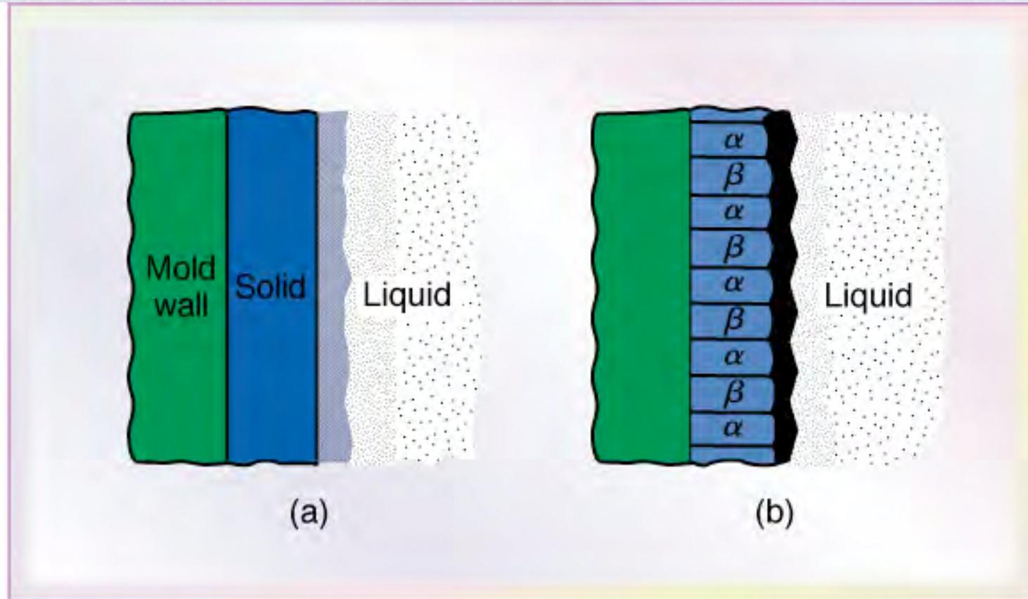
Figure 10.7 Schematic illustration of cast structures in (a) plane front, single phase, and (b) plane front, two phase. *Source:* Courtesy of D. Apelian
