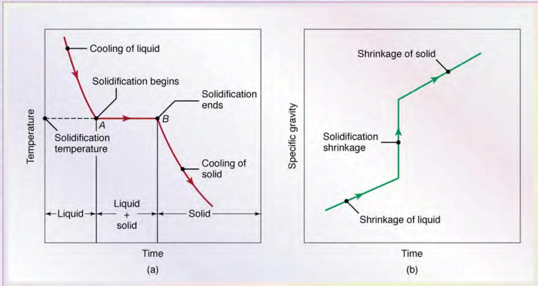
Figure 10.1 (a) Temperature as a function of time for the solidification of pure metals. Note that the freezing takes place at a constant temperature. (b) Density as a function of time
