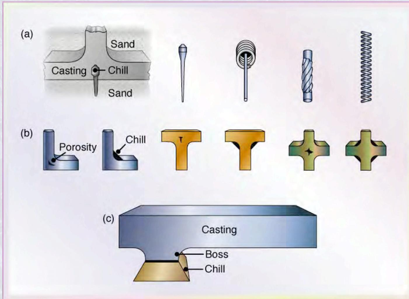
Figure 10.14 Various types of (a) internal and (b) external chills (dark areas at corners) used in castings to eliminate porosity caused by shrinkage. Chills are placed in regions where there is a larger volume of metal, as shown in (c).
