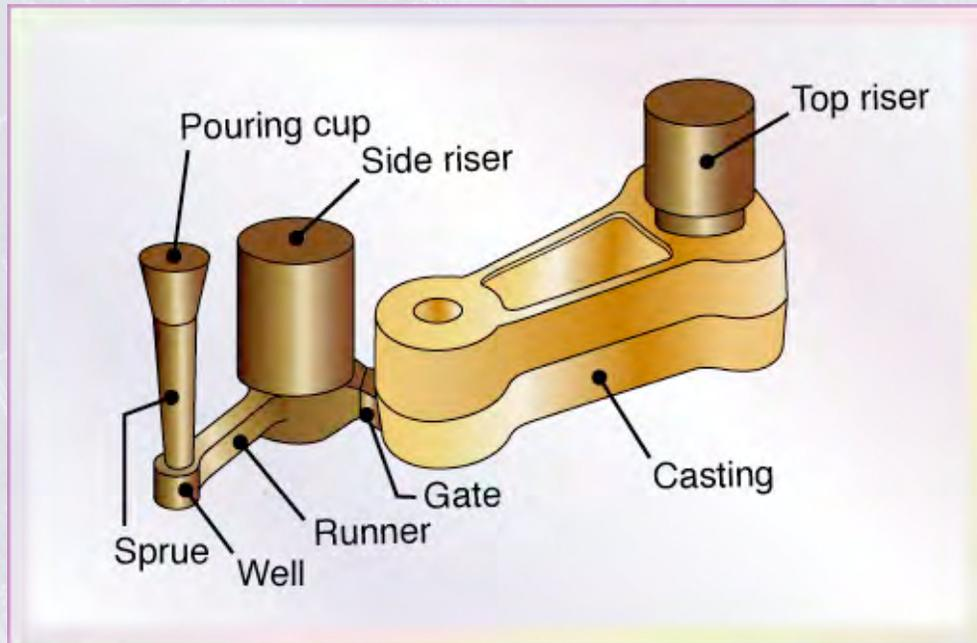
Figure 10.8 Schematic illustration of a typical riser-gated casting. Risers serve as reservoirs, supplying molten metal to the casting as it shrinks during solidification.
