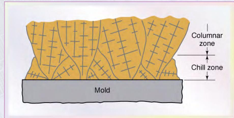
Figure 10.3 Development of a preferred texture at a cool mold wall. Note that only favorably oriented grains grow away from the surface of the mold
