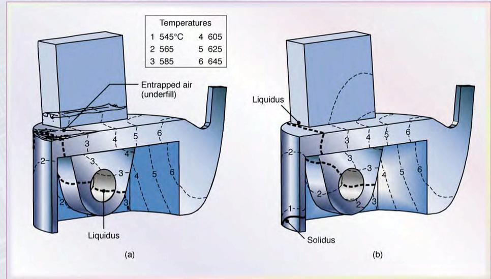
Figure 10.17 Simulation of mold filling and solidification. (a) 3.7 seconds after start of pour. Note that the mushy zone has been established before the mold is filled completely. (b) Using a vent in the mold for removal of entrapped air, 5 seconds after pour.
