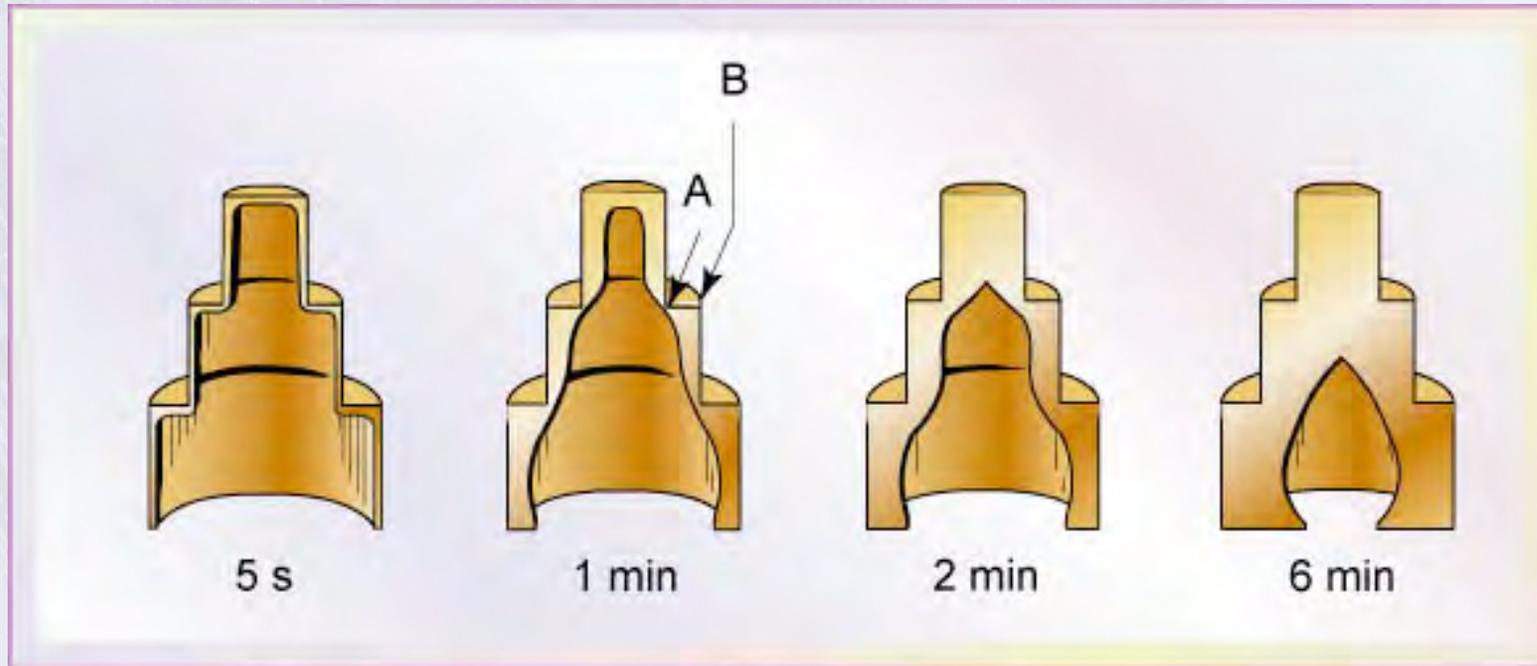
Figure 10.11 Solidified skin on a steel casting. The remaining molten metal is poured out at the times indicated in the figure. Hollow ornamental and decorative objects are made by a process called slush casting, which is based on this principle. *Source:* After H. F. Taylor, J. Wulff, and M. C. Flemings
