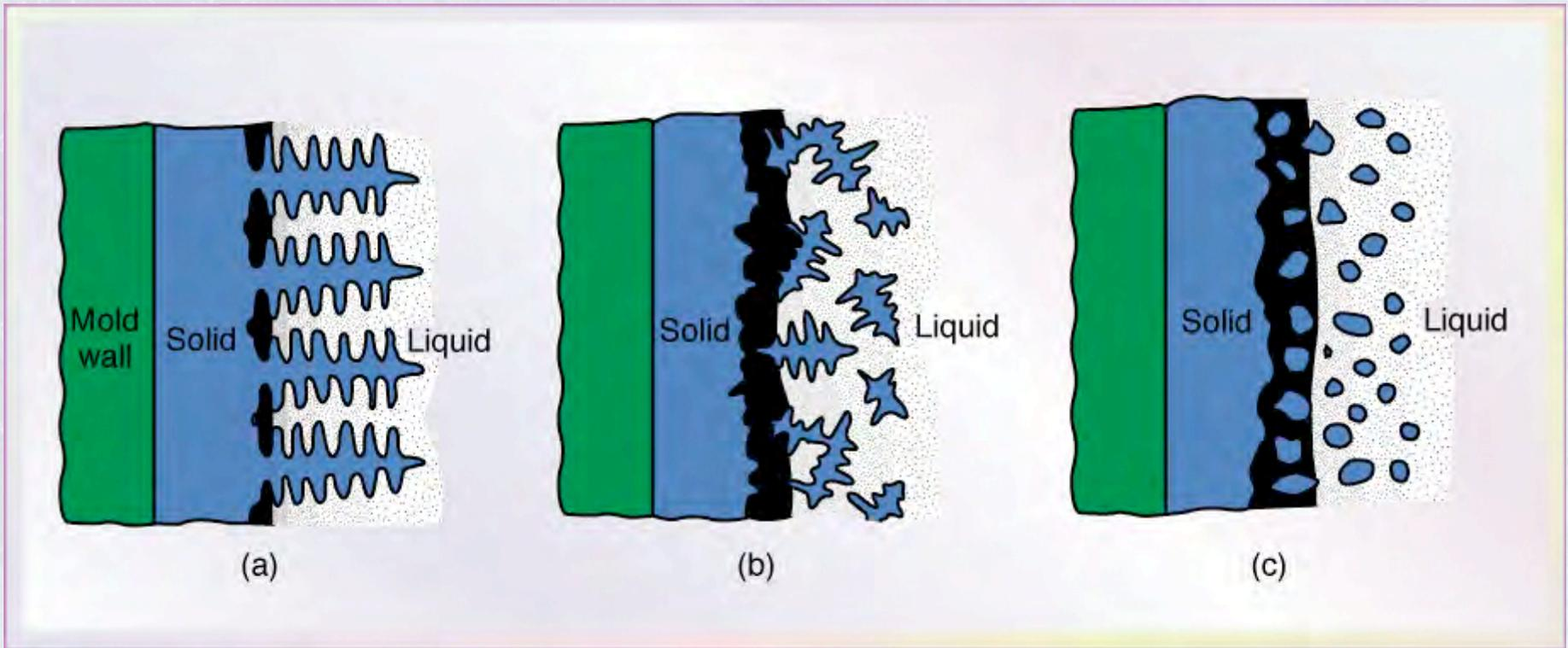
Figure 10.6 Schematic illustration of three basic types of cast structures: (a) columnar dendritic; (b) equiaxed dendritic; and (c) equiaxed nondendritic. *Source:* Courtesy of D. Apelian
