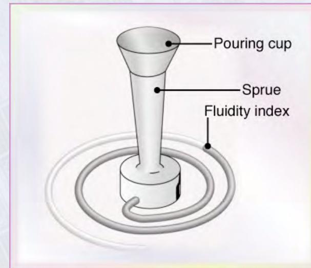
Figure 10.9 A test method for fluidity using a spiral mold. The *fluidity index* is the length of the solidified metal in the spiral passage. The greater the length of the solidified metal, the greater is its fluidity.
