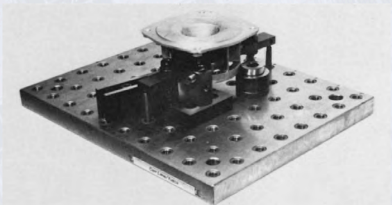
Figure 37.29 Completed modular fixture with cast-iron housing in place, as would be assembled for use in a machining center or CNC milling machine. Source: Courtesy of Carr Lane Manufacturing Company.
